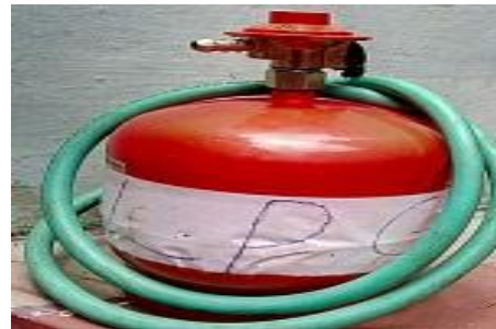
Fig: 1.2 LPG REGULATORS WITH HOSE PIPES
