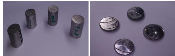
Fig 3: Compression test specimens (before and after t
