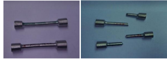
Fig 2: Tensile test specimens (before and after testing)
