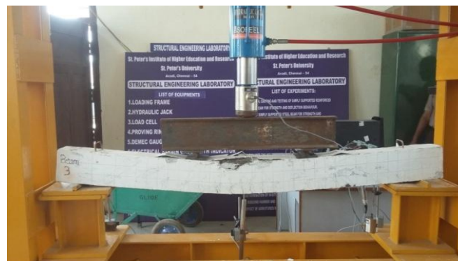
Fig -6: Beam after Failure
