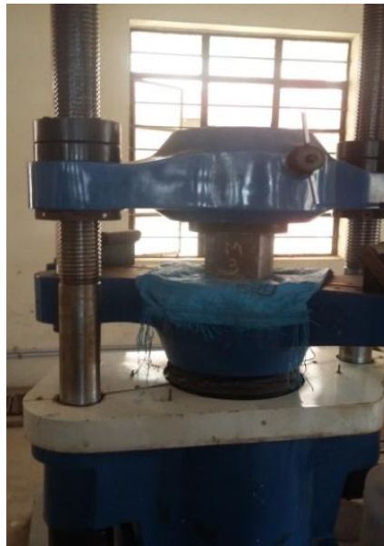
Fig-7: Testing of cube
