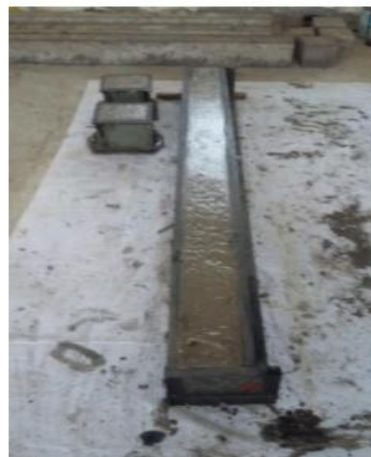
Fig- 3: Casting of beam specimens – Wet concrete in the mould
