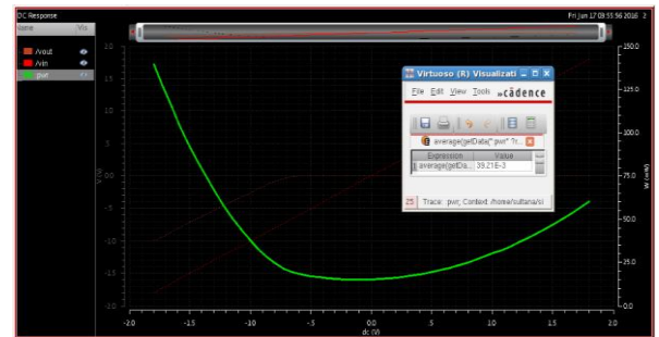
Figure 8: Short circuit power of LDO
