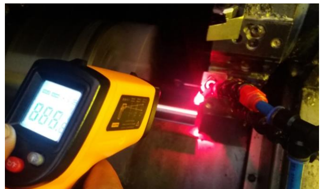
Fig -3: Avg. tool-chip interface temperature measurement
