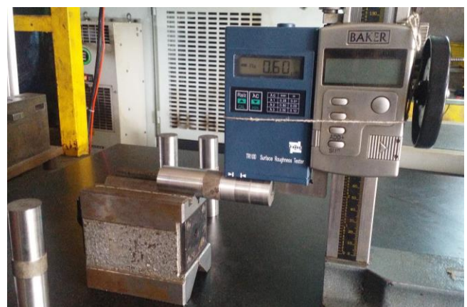
Fig -4: Testing of surface roughness (Ra)
