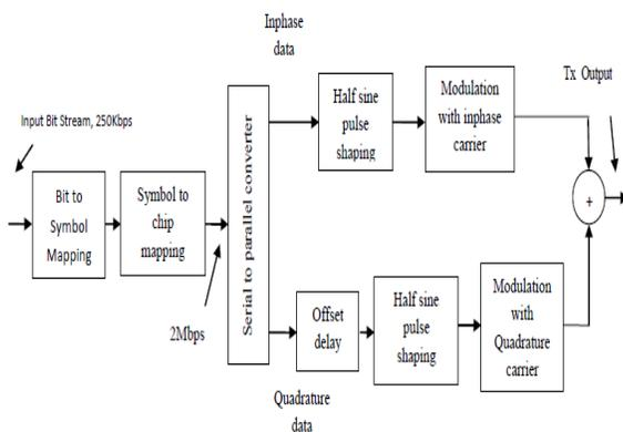
Fig 1.1 Block Diagram of ZigBee
