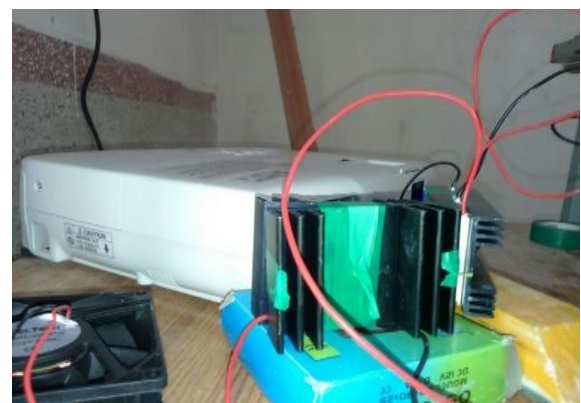
Fig 7: Three TEG modules in series
