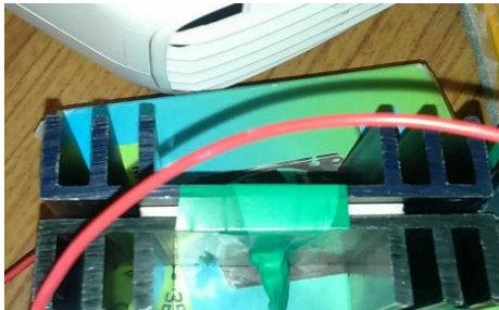
Fig 4: TEG with heat sink on both sides
