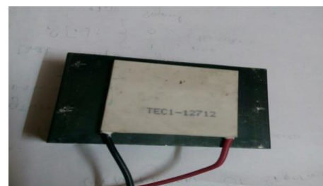
Fig 3: TEG with heat sink on one side
