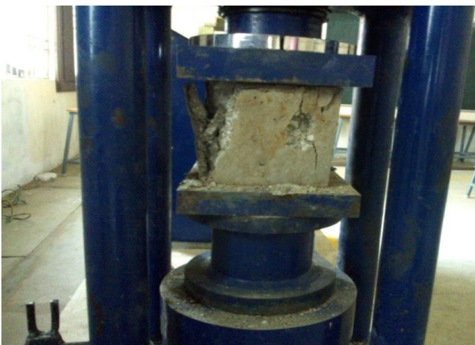
Fig -1: Testing of cubes for Compressive strength
