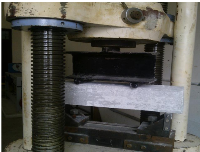
Fig -3: Testing of prisms for Flexure strength
