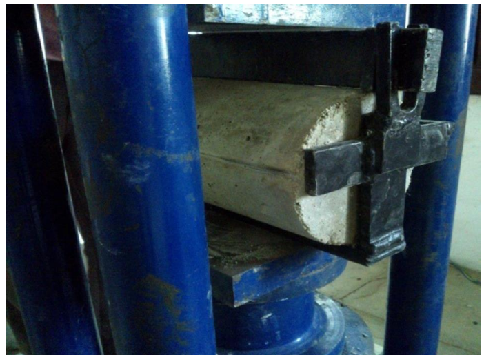
Fig -2: Testing of cylinders for Split tensile strength
