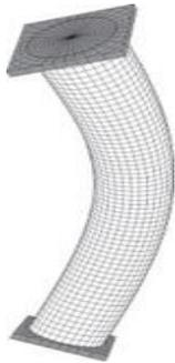
Buckling mode (Eigenmode 1) for concretefilled stainless steel tubular columns.
