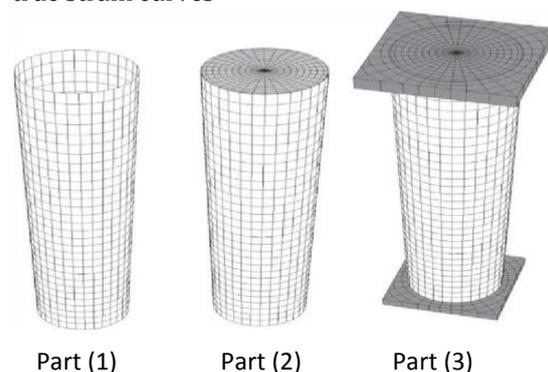
Modelling steps of concrete-filled stainless steel tubular columns. Part (1) Modelling of circular tubes using shell elements, Part (2) Modelling of concrete using solid elements and Part (3) Modelling of loading plates using solid elements
