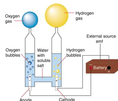
**Fig -5:** Experimental setup of electrolysis of water [12]
