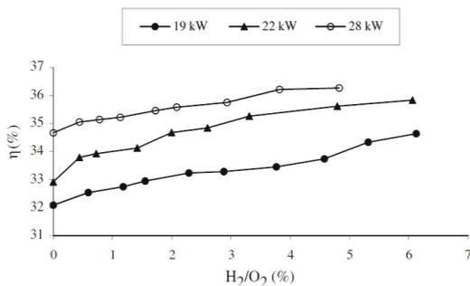
**Fig -1:** Variation of brake thermal efficiency with electrolysis product percentage [8].
