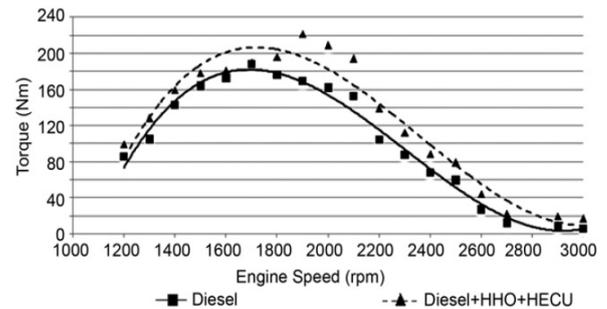
**Fig -3:** Variation of engine torque with engine speed [9].
