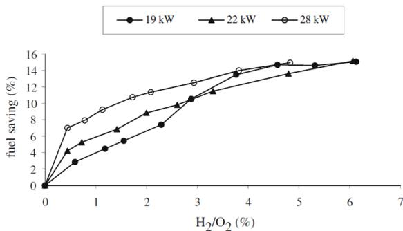
**Fig -2:** Variation of fuel saving with electrolysis product percentage [8].
