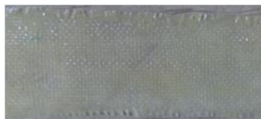
1 Layer of GFRP (Bi- directional)
