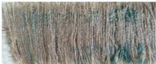
3 Layer natural fiber (Uni-Directional 0 degree)
