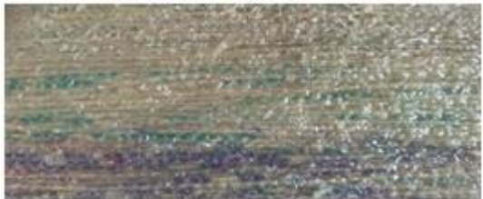
4 Layer natural fiber (Uni-Directional 0 degree)
