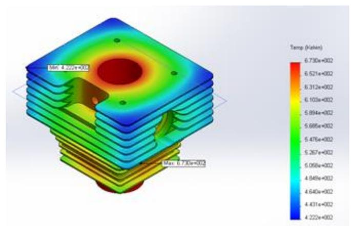
Fig5.1 Analysis of the model without notches
