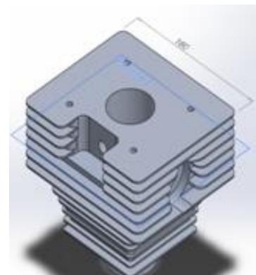
Fig4.1 Solid Model of Engine Block without notch
