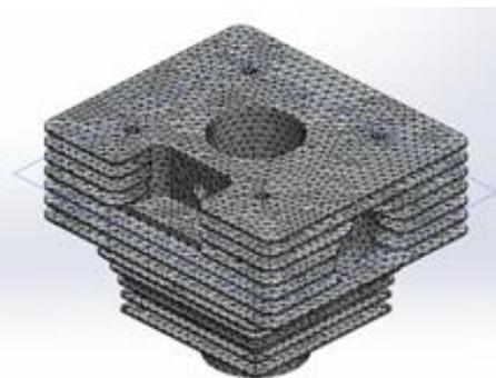
Fig4.3 Meshed model without notch
