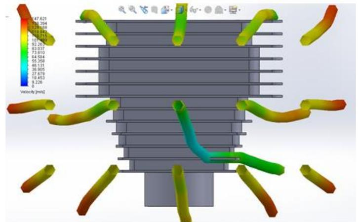
Fig4.5 Flow express of air over engine block
