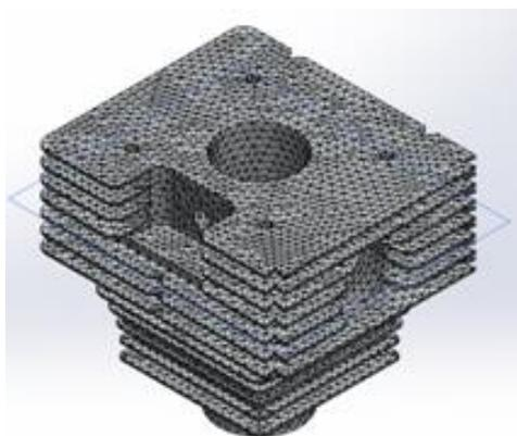
Fig4.4 Meshed model with notch
