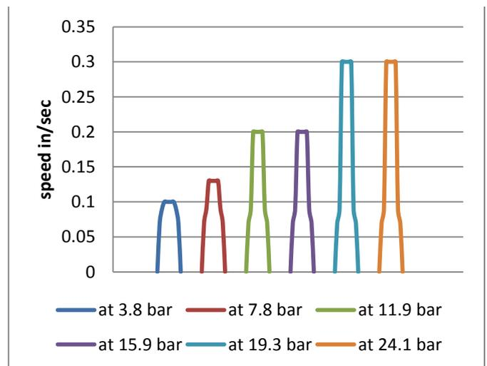
Fig -7 linear speed of hydraulic cylinder with 10% command value
