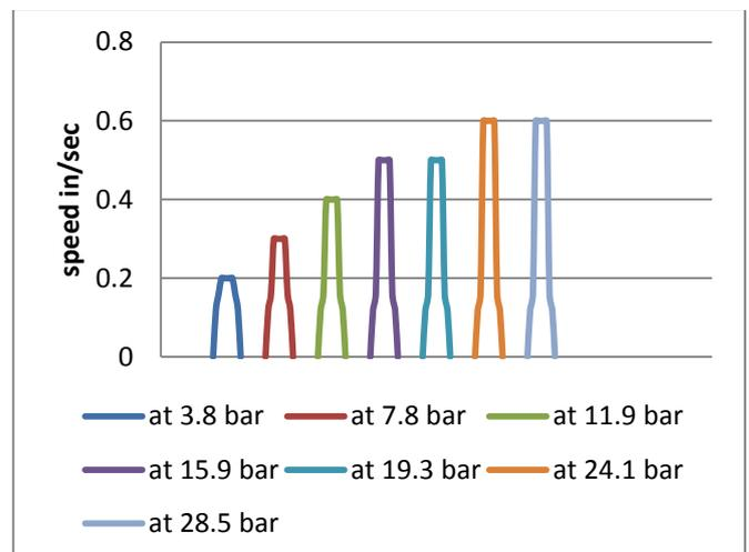
Fig -8 linear speed of hydraulic cylinder with 20% command value
