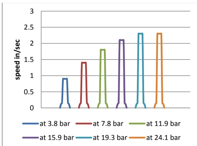
Fig -10 linear speed of hydraulic cylinder with 40% command value
