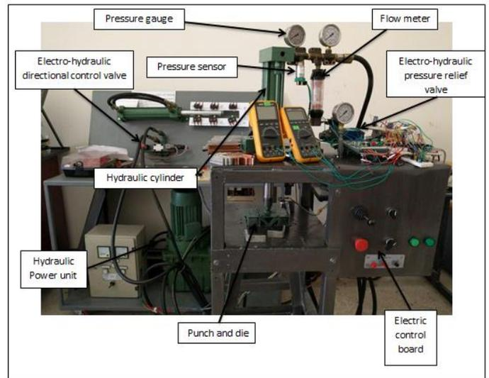
Fig -2: The Electro-hydraulic press machine system
