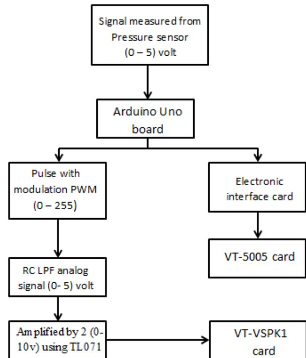
Fig -4: Block diagram of electronic circuit
