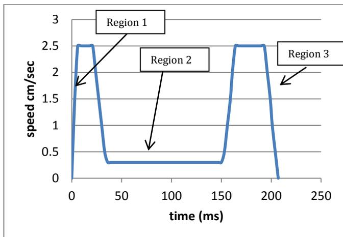
**Fig-14** press stroke speed of the system during bending
