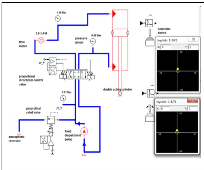
Fig -4: the simulation process of the electro hydraulic control system of the press machine
