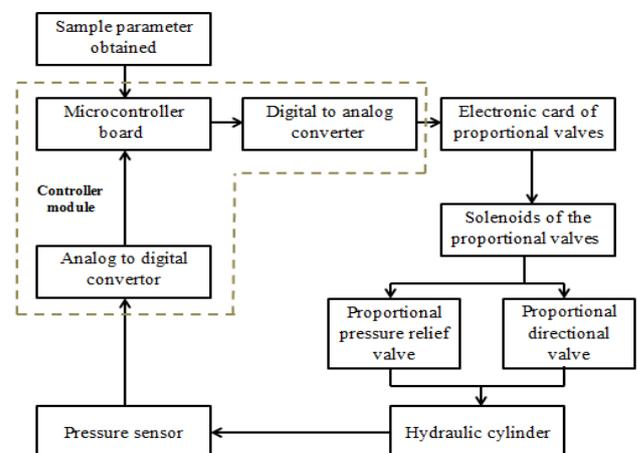
**Fig -1:** block diagram of proportional control system for speed and force controlling
