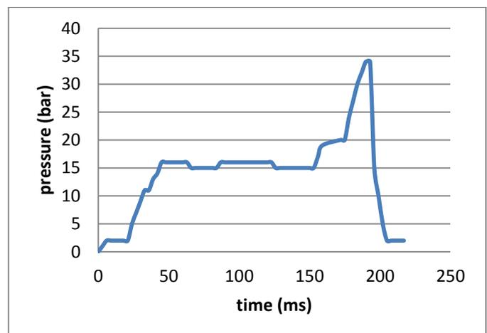
**Fig-13** system pressure behavior while bending copper alloy 5 mm thickness
