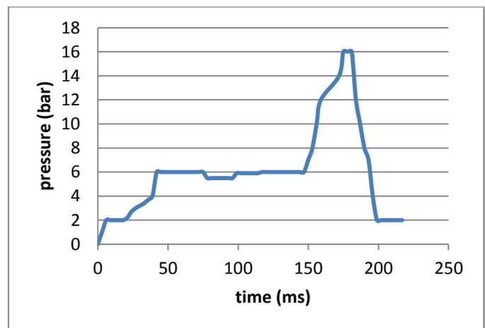
**Fig-12** system pressure behavior while bending copper alloy 3 mm thickness
