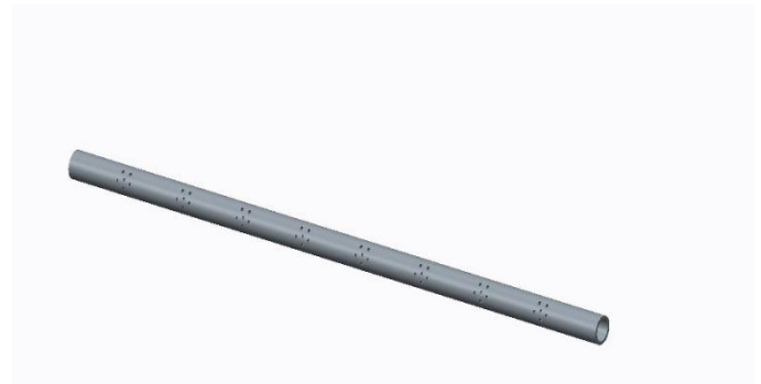
Fig.7: 3-Dimensional view of sprinklers containing pipe
