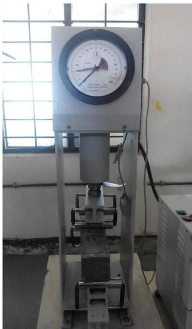
Fig -3: Flexural test setup
