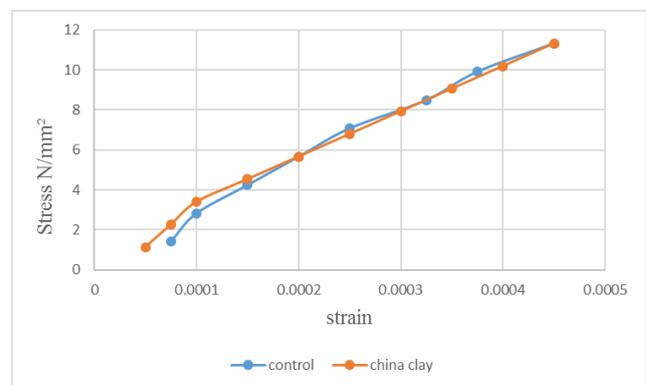
Chart -4: Combined stress strain curve for control and china clay
