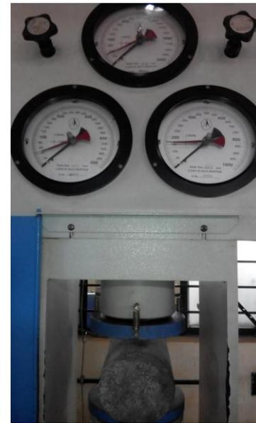
**Fig -2:** Split tensile test setup
