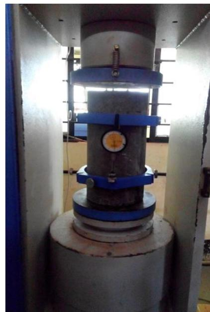
Fig -4: Modulus of elasticity test setup
