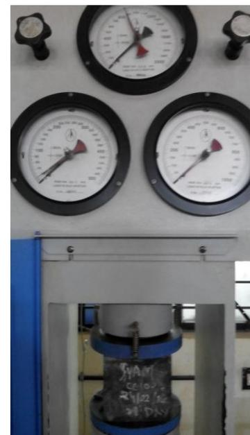
**Fig -1:** compression test setup
