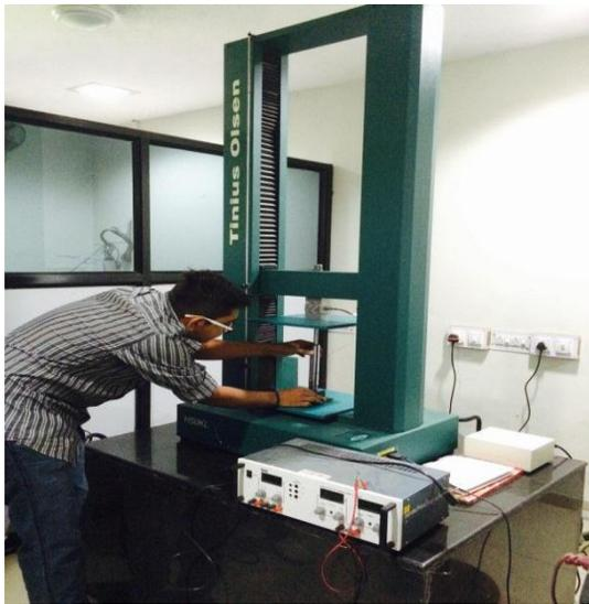
Fig.3 Tensile Test Machine & Constant Current Source Machine
