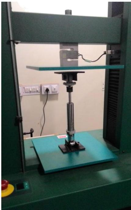
Fig.5 Suspension placed on test bench with mountings
