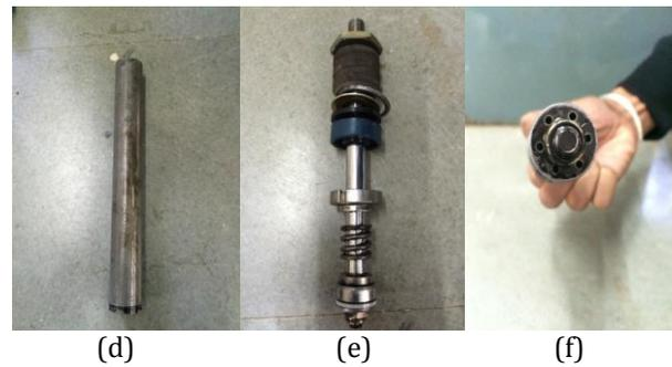
Fig 1 Shows the various parts of the Suspension: (a) Twin tube suspension, (b) Damper, (c) Outer cylinder, (d) Inner cylinder, (e) Piston and piston rod, (f) Valves with orifice
