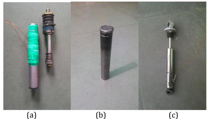
Fig.2 Shows the suspension after the modifications done on the original suspension (a) Solenoid wound over the inner cylinder, (b) Welded lower section of the inner cylinder, (c) Assembly of suspension with modifications.
