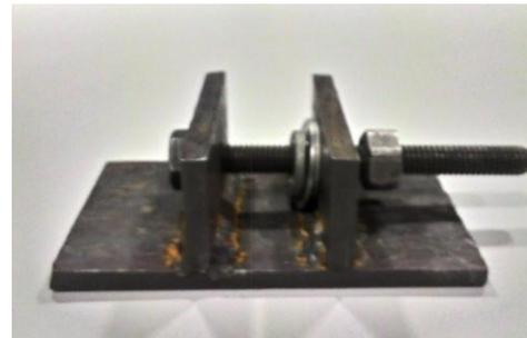
Fig.4 Fixture mounting used for suspension damper.
