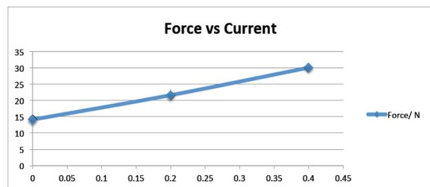
Fig.9 Force vs. current graph.
