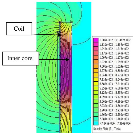
Fig.6 Asymmetric mode of MR damper in FEMM
