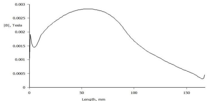
Fig.7 Variation of magnetic flux with length at 0.2A current
