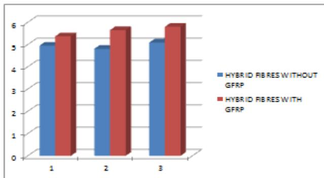
From the above graph the normal mix with grfp have increased by 4.61% and for fibre added concrete by 12% when compared to without grfp
