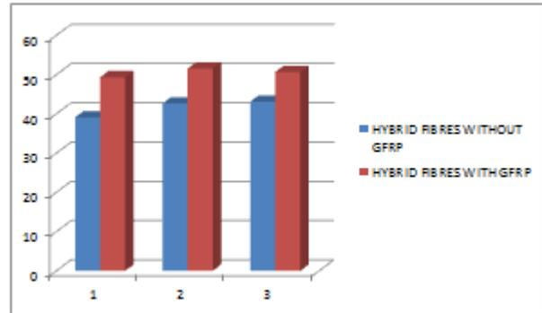
From the above graph the normal cube result increased for GFRP wrapping by 8.10%. and for hybrid concrete by 8.9Mpa when compared to without gfrp
