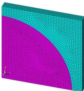
Figure 6: Converged Mesh Model of FRP Composite at 60 Vol. %
