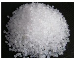
Figure 1: Polypropylene (granules)
