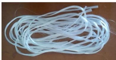
Figure 3: Continuous Glass Fiber
