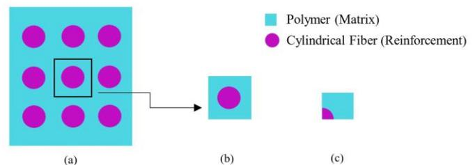
Figure 4: (a) Uniform distribution of fibers in matrix, (b) Isolated Unit cell and (c) One eighth Model
