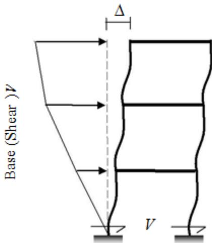
Fig: Schematic representation of pushover analysis procedure
