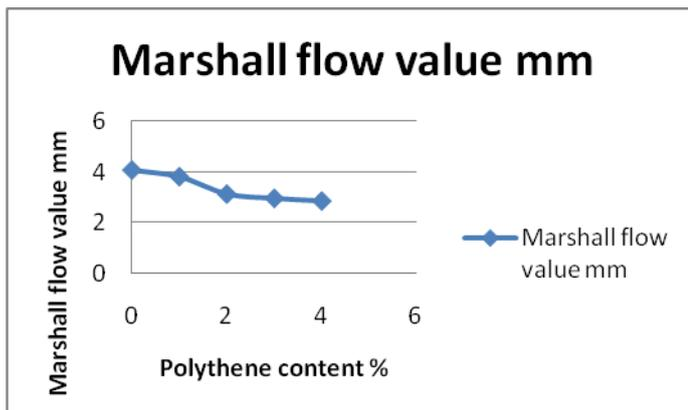
**Figure-3:** Marshall flow value vs. Polythene content
