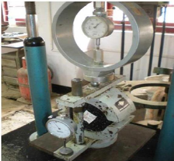
Figure-1: Marshall Test in progress
