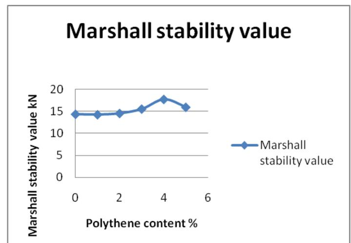
Figure-2: Marshall Stability value vs. Polythene content
