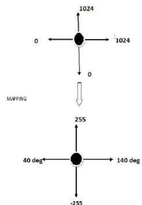
The analog data ranging from 0 to 1024 is read from joystick. Now the data is mapped to desired value as shown in figure. Convert the speed and direction values to char array. Now transmit the value through RF transmitter. Now wait till the whole message is sent.
