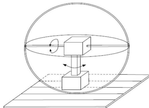
ROSPHERE has an inner two degrees-of-freedom pendulum. Figure 4.1 shows a general concept of the mechanism, including its main parts:
