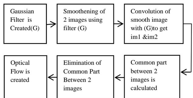
In Fig-2 Optical Flow determination is shown.
