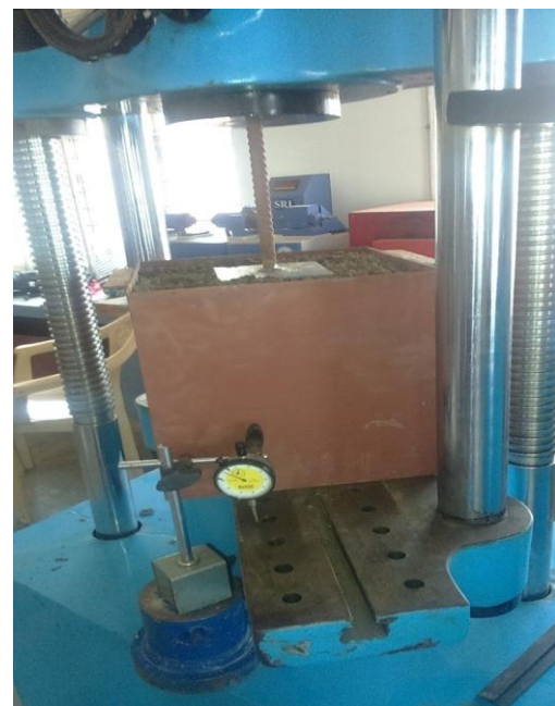
Fig 1.0 Experimental setup with a square tank and dial gauge
