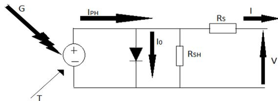
Figure 1: Single diode model of a solar cell [9]
