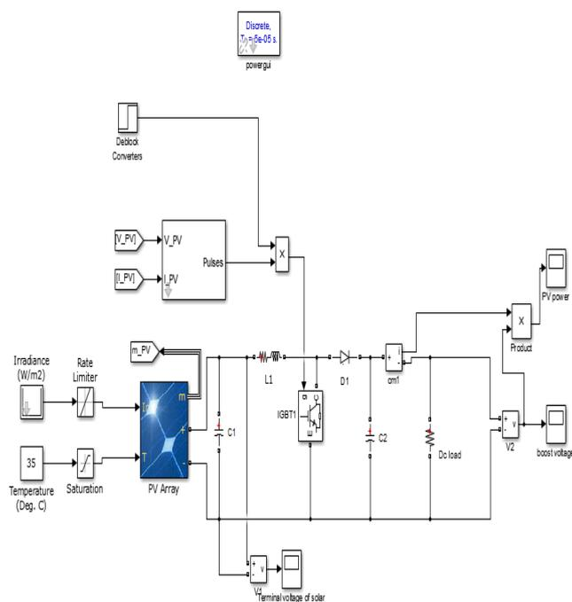
Fig: simulation of pv array using mppt.
