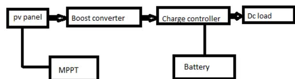
**Fig:** Electric generation from off grid system.
