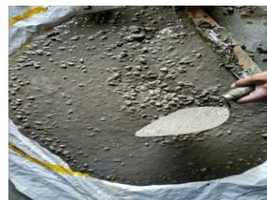
Fig.7- Mixing of self-compacting geo polymer concrete
