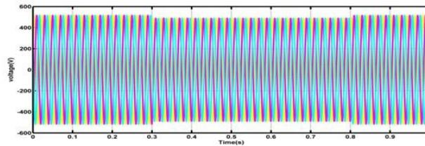
Fig.12. Voltage at PCC Without STATCOM
