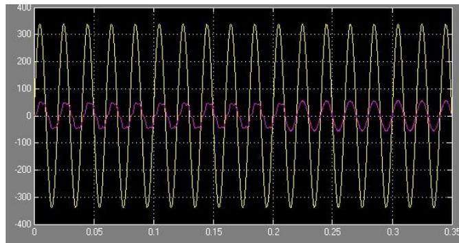
Fig.16. Supply Voltage and Current at PCC
