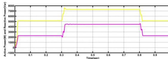
Fig.14 Active and Reactive Power Without STATCOM
