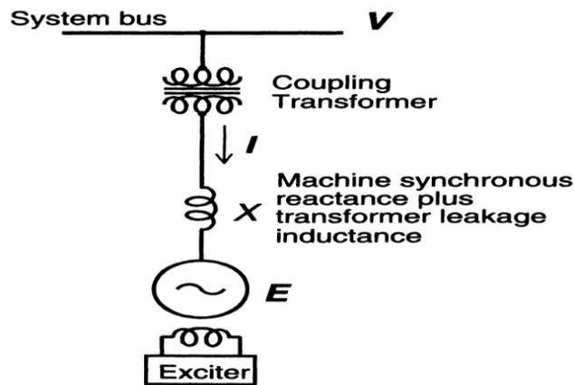
Fig. 2. Basic Principle of STATCOM
