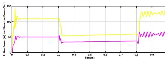
Fig.17. Active and Reactive Power With STATCOM
