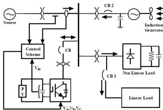
Fig.3. Schematic Model of System Operation of STATCOM Connected to Grid
