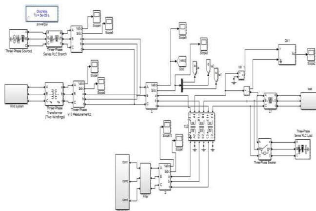
Fig.11.Diagram of Grid Integrated Wind Energy System using STATCOM
