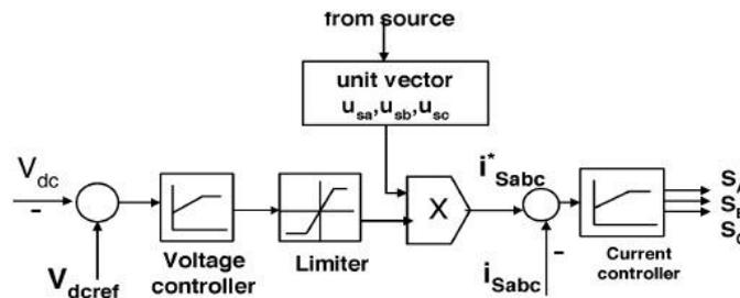
Fig.6 Control Scheme of STATCOM
