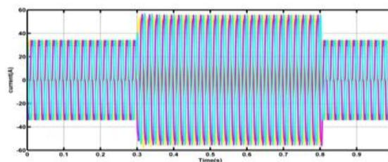
Fig.13.Current at PCC Without STATCOM
