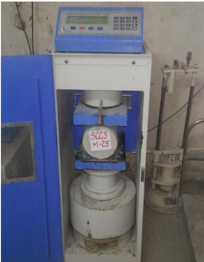
Fig -2: Split Tensile Strength Test Set up
