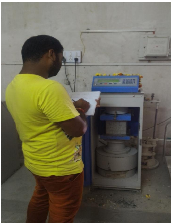
Fig -2: Compressive Strength Test Set up
