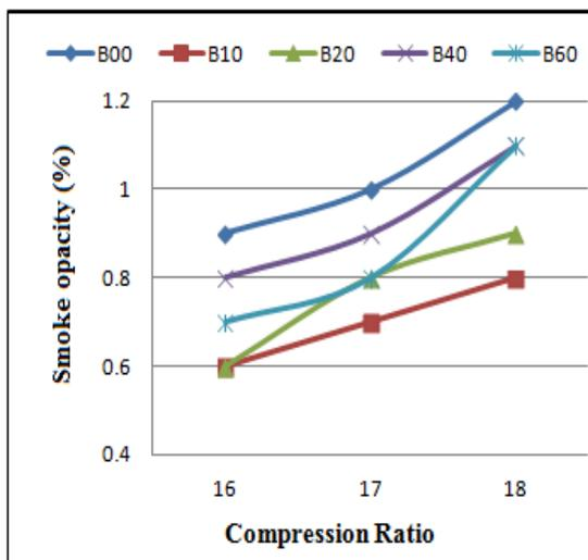
Figure 7: Variation of Smoke Emission with Compression Ratio.
