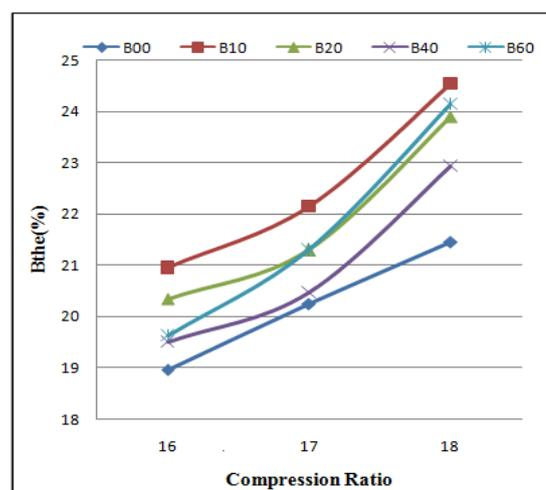
**Figure 2:** Variation of Brake Thermal Efficiency with Compression Ratio.
