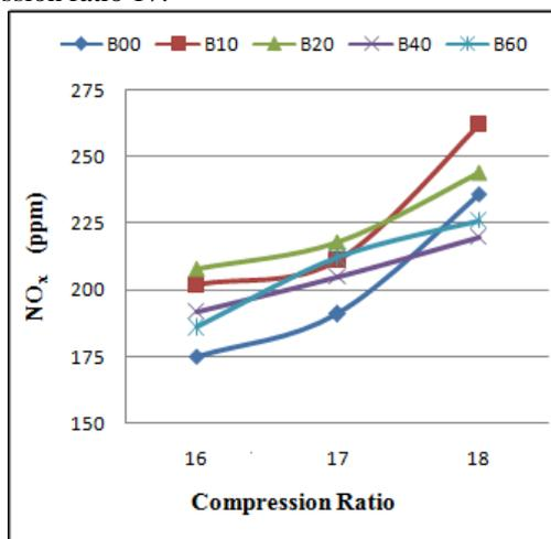
Figure 6: Variation of NO<sub>x</sub> Emission with Compression Ratio
