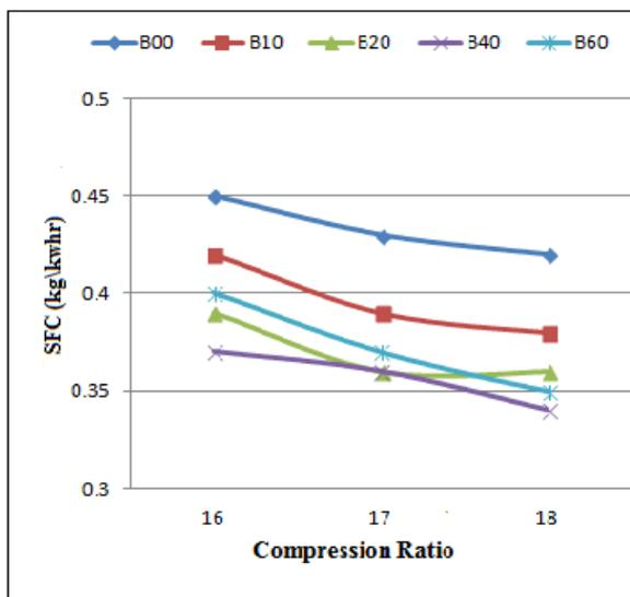
Figure 3: Variation of Specific fuel consumption with Compression Ratio.
