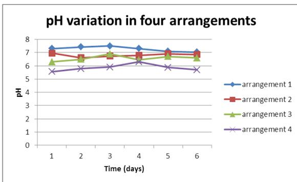
Fig 4.6: Graph depicting the variation in pH of filtered water in four arrangements
