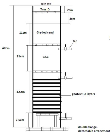
Fig 1.1: Schematic representation of column setup
