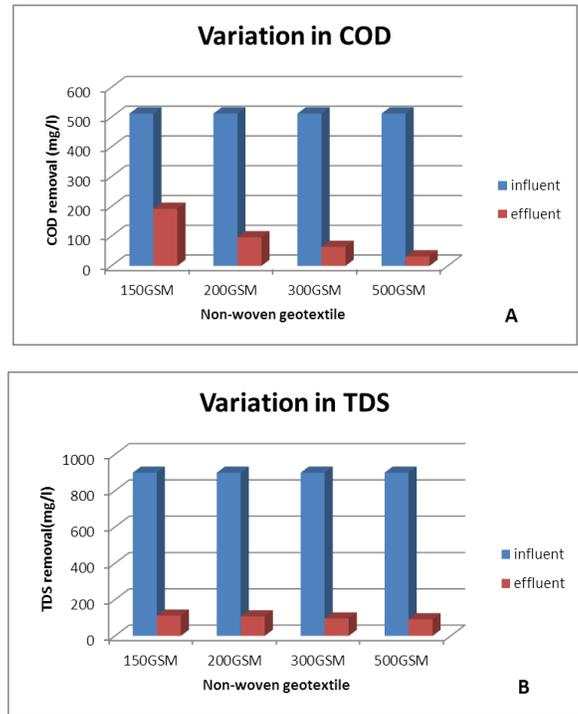
Fig 4.3(A) and (B): Graph showing the variation in COD and TDS after filtering through non-woven geotextile
