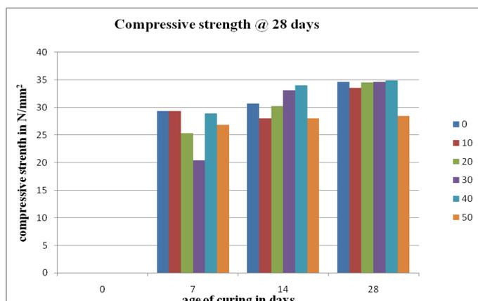
**Figure 1.** Compressive strength versus age
