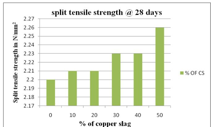
**Figure 2.** Split Tensile Strength versus % of Copper slag
