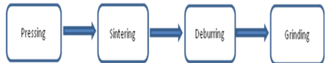
Figure 1: Process Flow (Before Kaizen)
