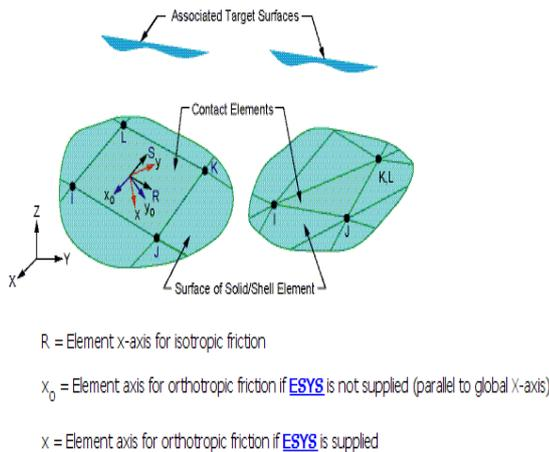
**Fig.3: CONTACT173 Element**
