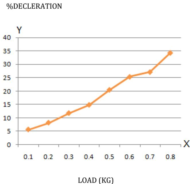
Figure 13:graph of percentage deceleration vs brake load
