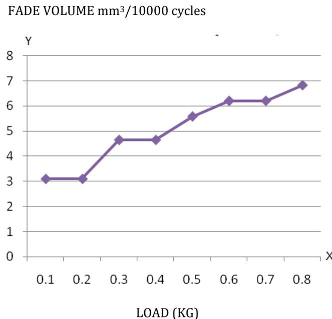
Figure 14:graph of fade volume/ 10000 cycles vs brake load
