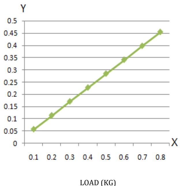
Figure 12: graph of brake torque vs brake load
