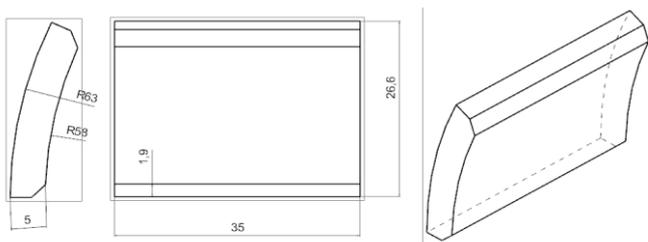
Figure 3: Geometry of discrete liner
