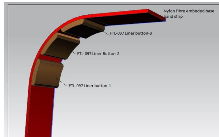
Figure 1: Discrete FTL-097 button liner
