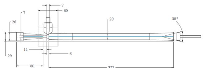
Figure 3.10 (j) Drafting of Vortex Tubes
