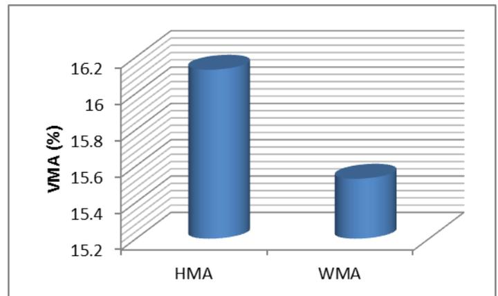
Figure 4.3: VMA (%) value comparison between HMA and WMA
