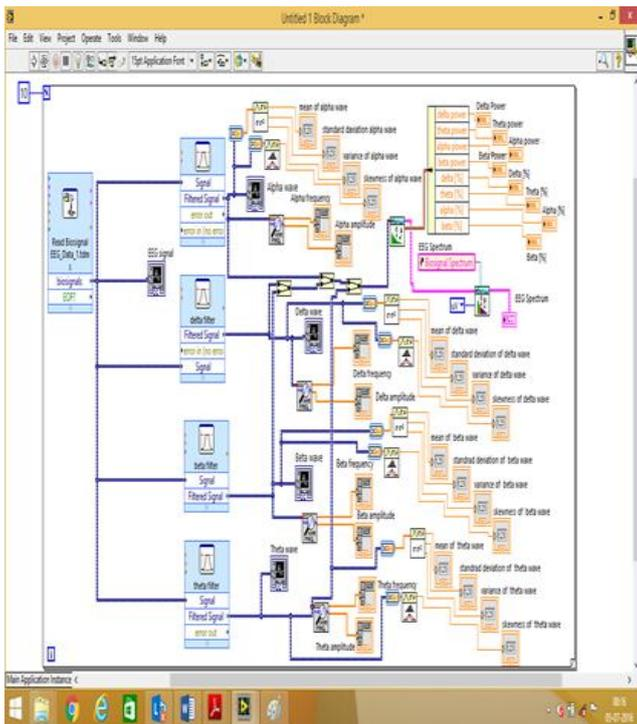
**Fig.5** FFT spectral analysis and feature extraction of EEG signal on lab view
