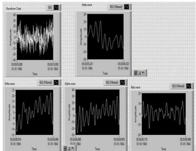
**Fig.7** Front panel of the original and filtered signal of diff. frequency band filters Alpha filter, Beta filter, Delta filter, and Theta filters
