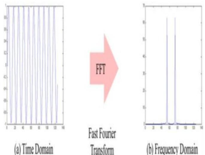
**Fig.4** Fast Fourier Transform
