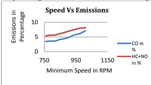
**Chart No-2:** Graphical representation of Speed Vs Emissions with Catalytic converter without Air-box.
