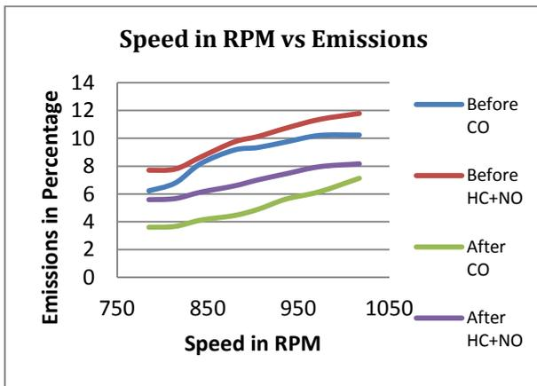
**Chart No-6:** Comparison of Emissions before and after using catalytic converter
