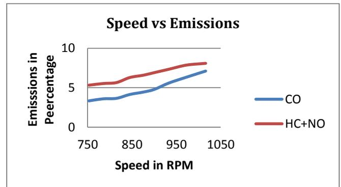
**Chart No-4:**Graphical representation of Speed Vs Emissions with Catalytic converter & Air box.
