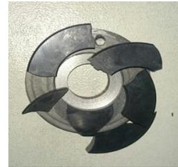
**Fig -11: Failure of thrust bearing (Formation of triangular area)**
