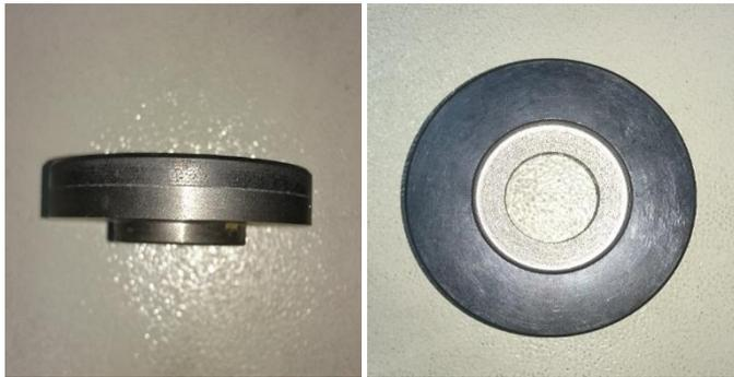
Fig - 1 Top view and front view of Carbon thrust bearing
