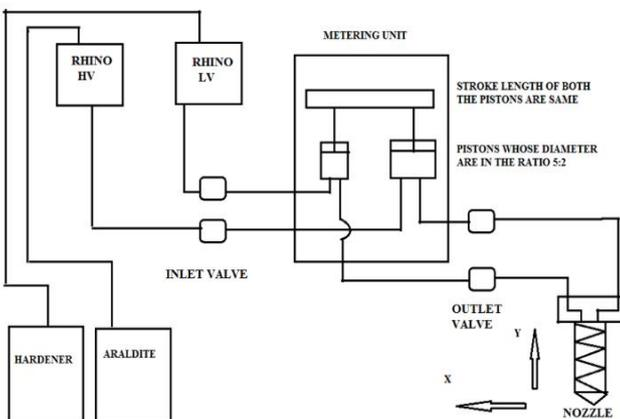
Fig -4: Simplified layout of Automatic bonding
