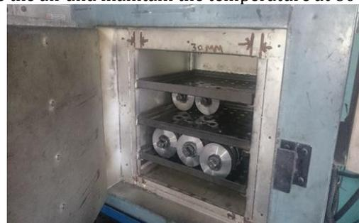
Fig -2: Oven for manual bonding
