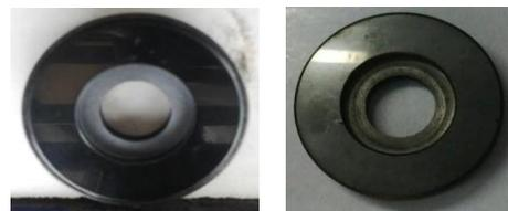
Fig-5: Before and after machining of thrust plate
