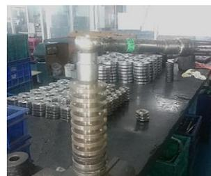
Fig -3: Mandrel with bearing tightened by torque wrench.
