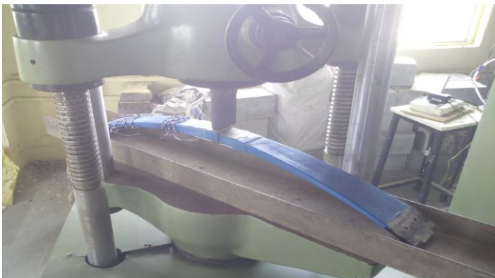
Fig-7: Experimental testing of composite leaf
