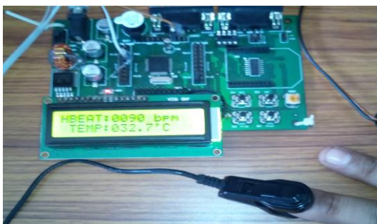
Fig 5.4: 30 0 -40 0 c temperature and Heart beat rating at Alert stat
