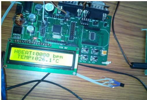
Fig 5.3 : 20-30 0 c temperature and Heart beat rating at Alert stat
