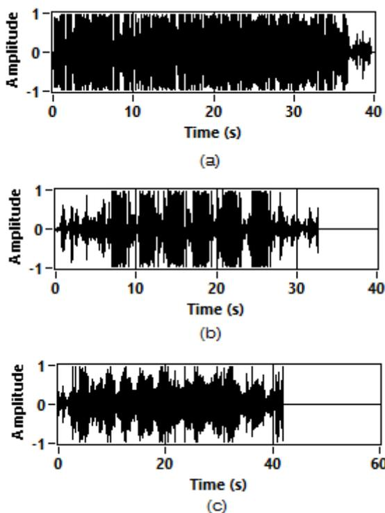
Figure 4. Sensed sound signals in time domain (a) healthy motor (b) motor with rotor fault (c) motor with eccentricity fault
