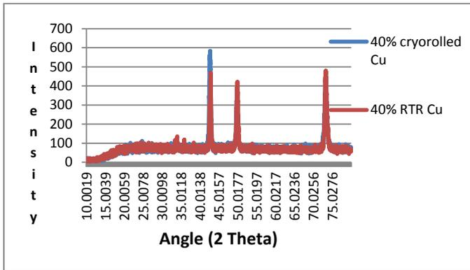
Chart 5: XRD test for 40% thickness reduction for Copper
