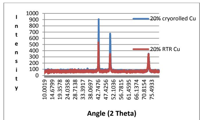
Chart 4: XRD test for 20% thickness reduction for Copper
