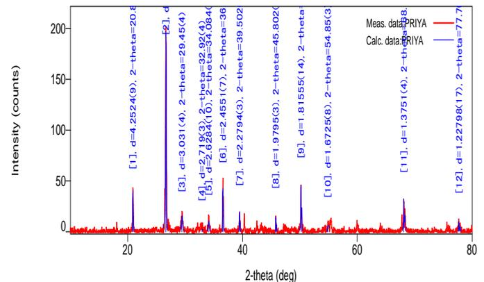
**Fig-2:** XRD analysis of specimen containing 10% of WFS.
