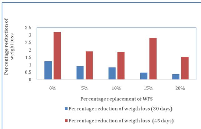
**Fig-5:** Weight loss due to sulphate attack when immersed in 5% solution of sodium sulphate.
