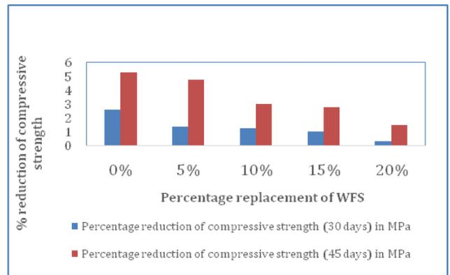
**Fig-3:** variation of compressive strength after sulphate attack immersed in 5% solution of sodium sulphate
