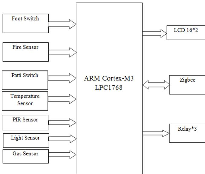
Figure1: Block diagram of proposed system at flat terminal
