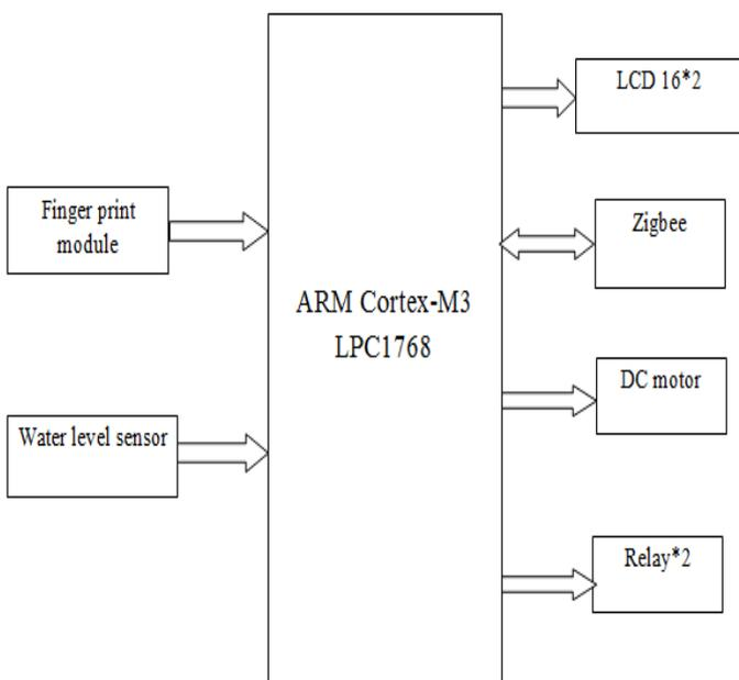
Figure 2: Block diagram of proposed system at society terminal.
