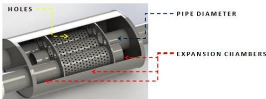
Fig 3 : Cut section and parameter of muffler
