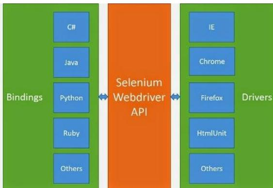
**Fig -2:** Architecture of Selenium Web Driver
