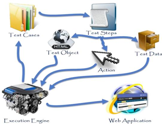
**Fig -4:** Architecture of Keyword Driven Approach
