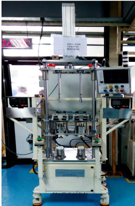
**Fig-2:** Dry Leak Testing Machine
