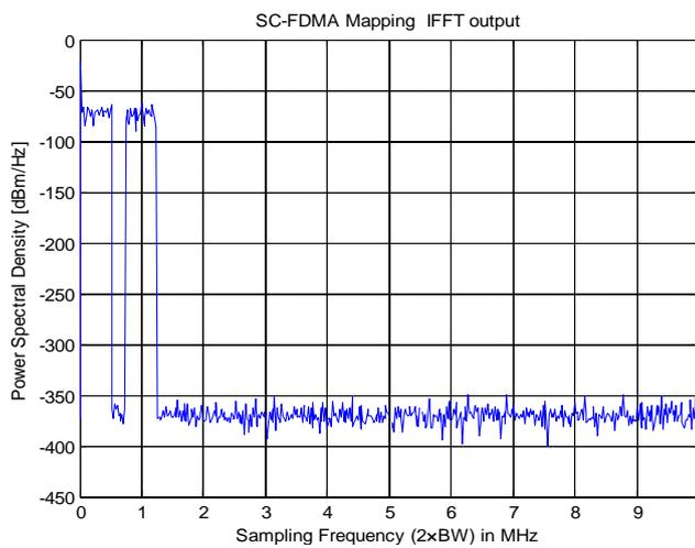
Fig -2: SC-FDMA signal IFFT output
