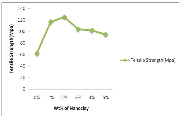
**Chart -1:** Tensile strength variations for different wt% of nanoclay
