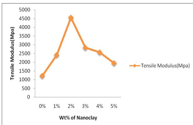
**Chart -2:** Tensile Modulus variations for different wt% of Nanoclay
