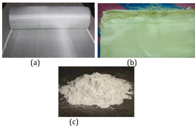
Fig -1: (a) S-glass fabric ,(b) Kevlar woven fabric, (c) Nanoclay
