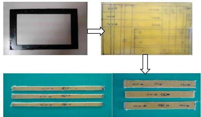
Fig- 1: Specimen preparation
