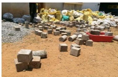
Fig.10- ambient curing of geo polymer specimens.
